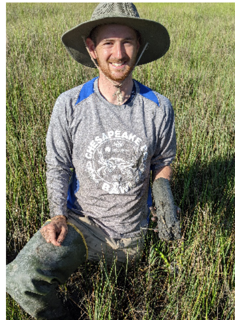
Root and soil core collected on Sapelo Island, Georgia, on 17 June 2021. After washing away the soil and separating live and dead roots, I am able to quantify root growth in the marsh
