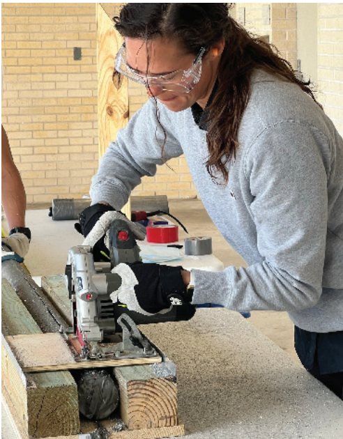
Cutting open a reef core using a custom cradle to reveal the internal structure of an oyster reef. Cores were collected with the help of T. Baker Smith LLC
